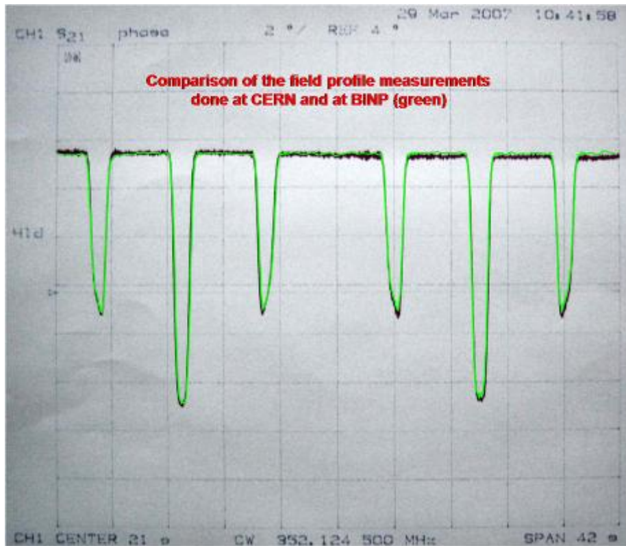
Figure 9 Bead-pull measurement of the CCDTL. The black trace corresponds to the measurement done at CERN, the green one to the measurement done at BINP
