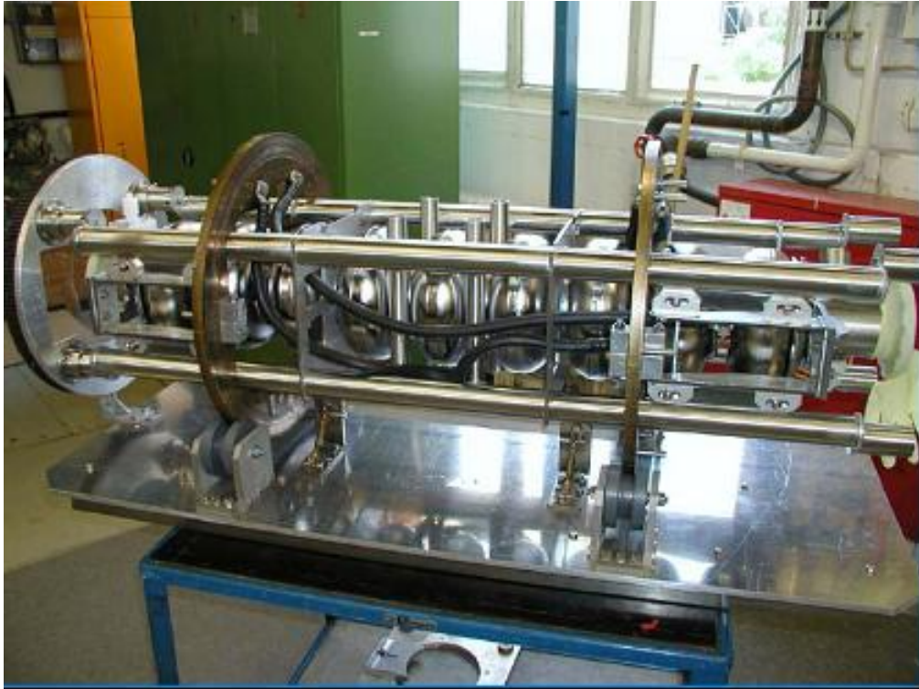
Figure 4 Details of the EP mechanical frame at DESY.
