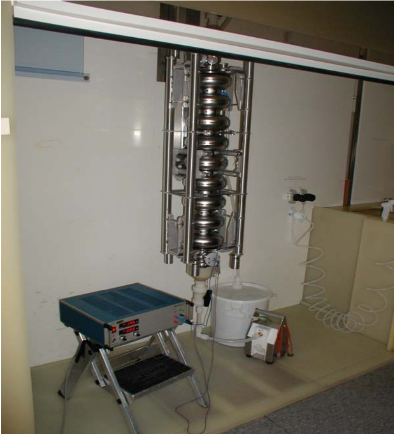
Figure 9: Test set up for anodisation of nine cell resonator inside the DESY cleanroom
