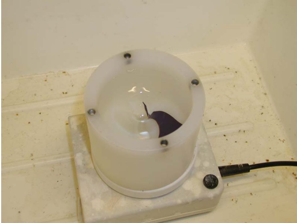
Figure 2: PVDF container filled with HF acid (4,8 % concentration). At the bottom the agitation driving unit can be seen
