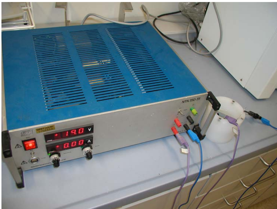
Figure 1: Test set up for oxidation of Niobium Samples Left side: power supply Right side: Teflon® container filled with HNO 3 (8% concentration)
