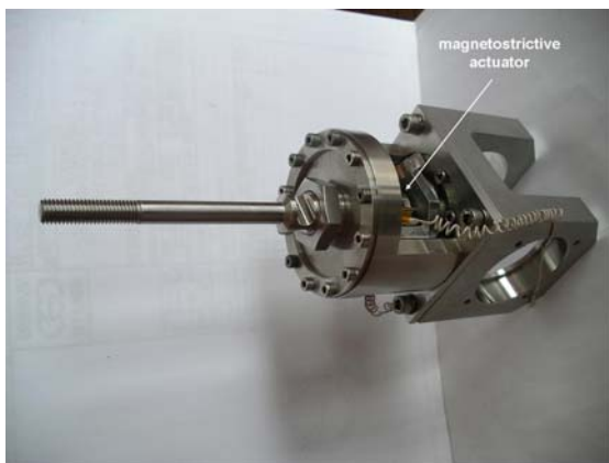
Figures 10: Modified mechanical part of the CTS for Magnetostrictive Actuator use (left); Integration on 9-cell cavity (right).
