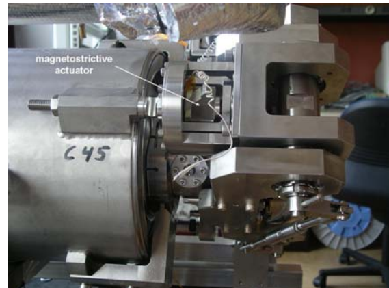
Figures 10: Modified mechanical part of the CTS for Magnetostrictive Actuator use (left); Integration on 9-cell cavity (right).
