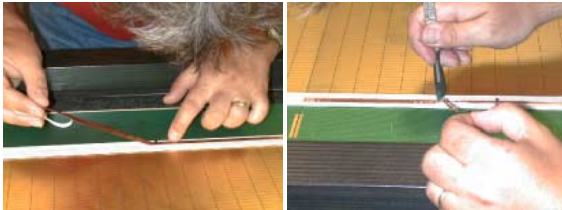
Figure 14: On the left, copper strip putting; on the right, copper strip cutting.
