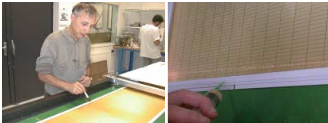
Figure 13: Wire cleaning (left) and glue putting on spacers (right) operations.
