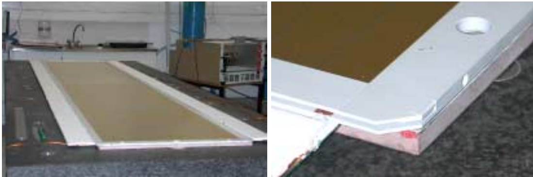
Figure 18: View of bending plane with non bending spacers positioned (left) and particular of corner (right).
