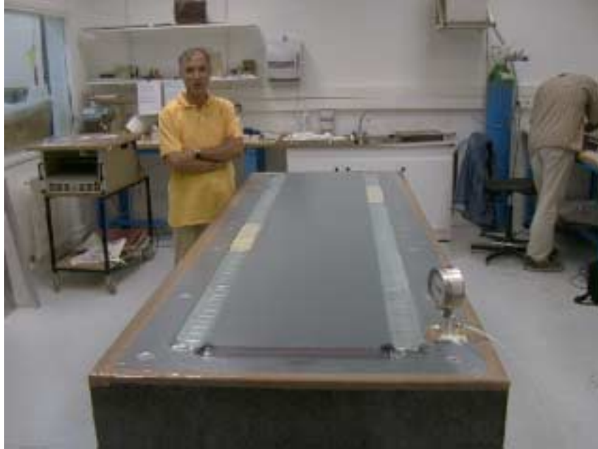
Figure 5: Polemerization completed under vacuum.
