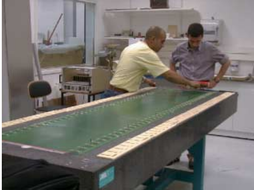
Figure 4: PCBs gluing procedure.
