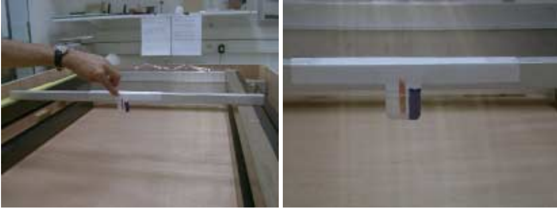
Figure 11: Wire tension check device.
