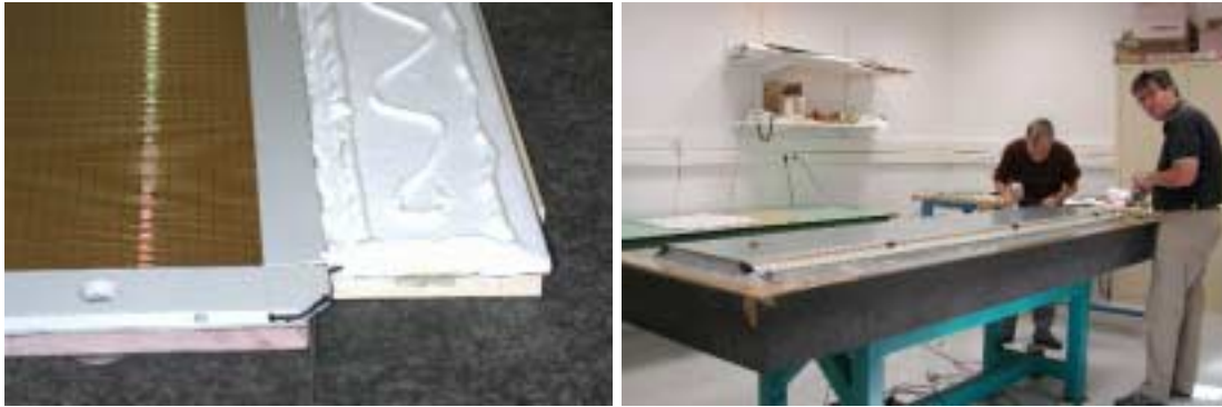
Figure 19: Particular of silicon spreading (left) and under vacuum closing operation (right).
