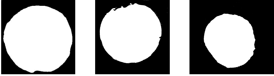
FIGURE 1. The binary image of the sample: white heat transfer area and black glued area. From the right hand side, 2mm, 3mm and 4mm sample. The heat transfer area is attributed to the white area.
