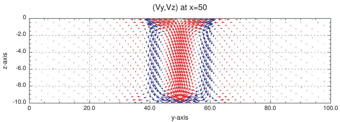
Fig. 2.— Velocity field used for the kinematic MHD model in  $\Omega_-$ . The velocity field is divergence-free and describes the motion in a main central convection cell and two closing external weak half-cells.
