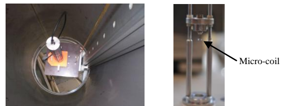
Fig. 1 NMR measurement pictures. Left, probe and shim stack mounted on the mechanical support. Right, micro-coil ( \varnothing=1.2 , 2.4 mm length) on base.
