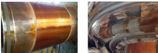
Fig. 6 Coil stabilization realization. Insert picture (left), FCL2 picture (right)
