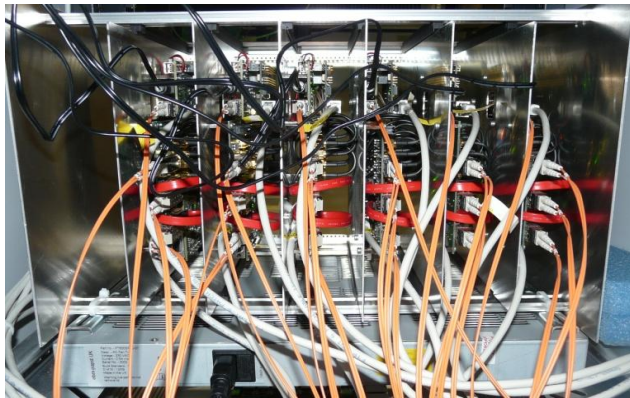
Fig. 4. Rear view of a custom-made crate populated with its six DCCs.
