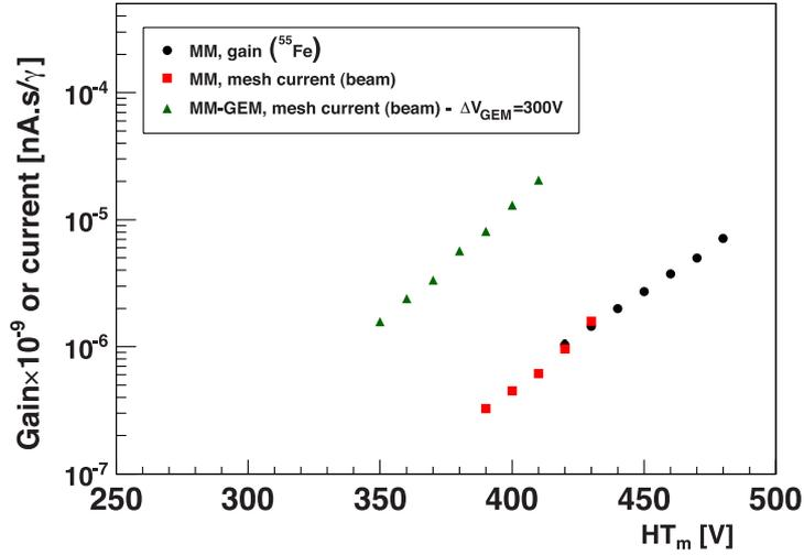
Figure 2: Gain measurements with a  $^{55}\text{Fe}$  source and mesh currents monitored during the tests for the 2 detectors. The comparison of the two measurements allows for the gain determination for the detector with the GEM foil.
