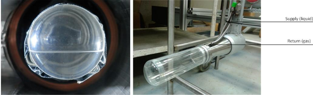
**Fig. 2.2** – (Left) Front view (from downstream) of the target during the filling phase. The liquid-gas interface of hydrogen is clearly visible. (Right) Front view of the target cell mounted on its aluminum support with the supply and exhaust tubes for hydrogen.
