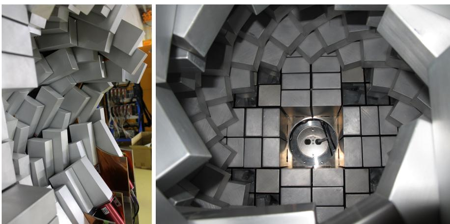
**Fig. 4.4** – Picture of the DALI2 gamma array. (Left) Half of the DALI2 crystals, seen from downstream, with the first layer crystals clearly visible. (Right) DALI2 crystals geometry shown from upstream. The last 11<sup>th</sup> layer of crystals is shown in the background.
