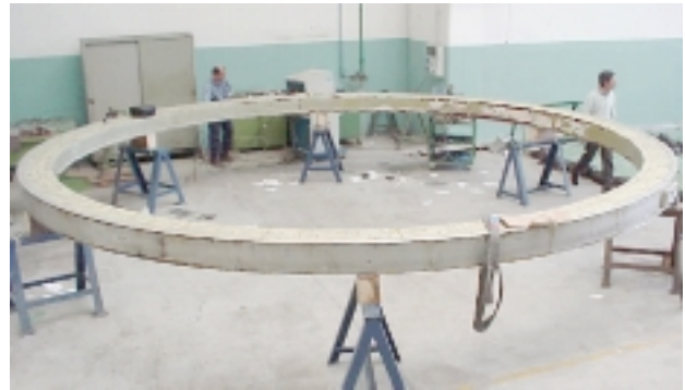
Fig. 9. The model coil extracted from impregnation mold.
