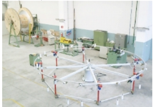
Fig. 5. Pre-bending operation. After spooling the conductor is straightened and bent. After bending the turns are stored on the large wheel.
