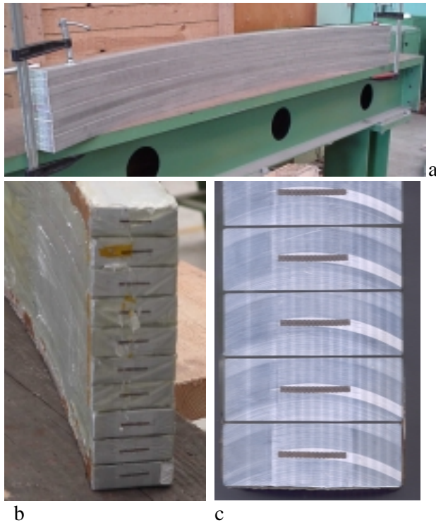
Fig. 4. One of the stacks during construction: (a) assembling phase, (b) after impregnation, (c) sectioned.
