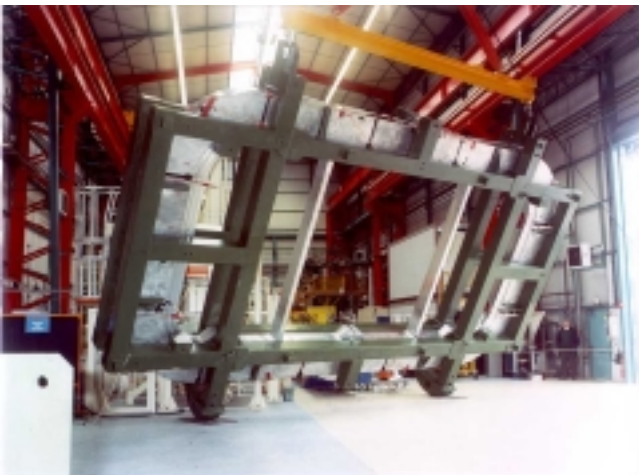
Fig. 4. Handling of the B0 Coil cold mass
