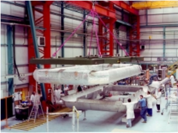
Fig. 8 View of the cold mass assembly in the lower half vacuum vessel
