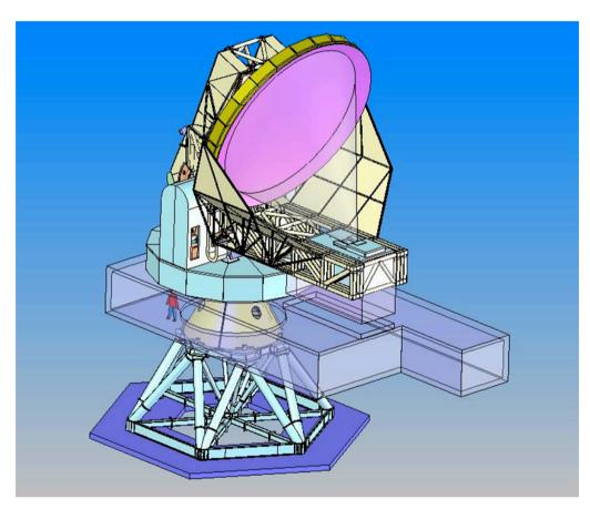
Schematic of the SPT, when Telescope is 'Docked' for access to the Receiver Cabin
