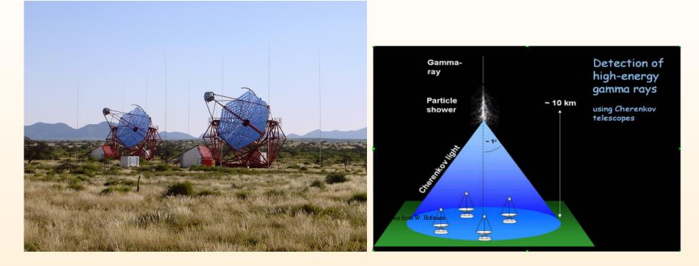
Čerenkov telescopes have huge effective areas (  $10^5m^2$ ), relatively good energy resolution ( 10%), PSF  $0.1^{\circ}$  but with a poor duty cycle (weather, moonless nights). The most constrained observatories in MWL campaigns.
