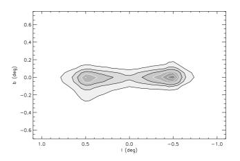
Fig. 9. Maximum entropy image in the 1173 keV  $^{60}$ Co line shows the capability of the instrument to separate sources closer than the angular resolution, where the signal-to-noise ratio is good. The sources are separated by  $1^{\circ}$ .
