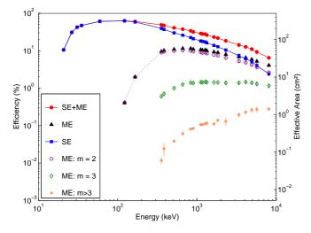
Fig. 4. Full-energy peak efficiency for SE, ME and all events (SE+ME) and for ME with multiplicity m = 2, 3 and > 3, for the camera without mask. The effective area is the geometric area multiplied by the efficiency.
