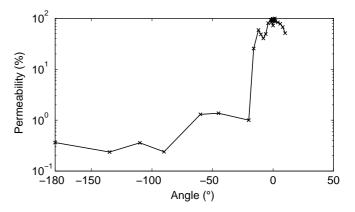
Fig. 11. ACS permeability as a function of the angle from the axis (BLC,  $^{137}$ Cs source)
