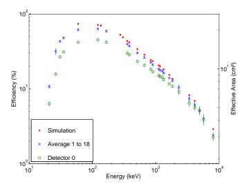
Fig. 2. Full-energy peak efficiency for sources on the SPI optical axis ( $\alpha = 0^{\circ}$ ), without mask. An average for detectors 1 to 18 is shown; detector 0 is plotted separately (see Sec. 5.2). The measurements are compared to Monte-Carlo simulations.
