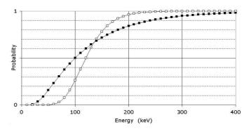
**Fig. 10.** For PMT<sub>1</sub>(solid),  $E_{\rm th} = 100$  keV and  $a = \sqrt{50}$ , for PMT<sub>2</sub>(open), 120 keV and  $\sqrt{10}$ . These curves illustrate the large differences between ACS crystals and PMTs combinations.
