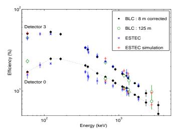
**Fig. 5.** The on-axis, full-energy peak efficiencies of detector 0 and 3 for SPI with its mask. The data are: 8 m BLC data without mask corrected for the mask absorption (·), 125 m BLC data with mask, (o) and 8 m ESTEC data with mask (×). For detector 0, the disagreement between the curves shows the difficulty of alignment device modelisation.
