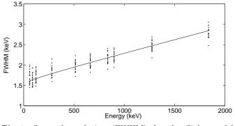
**Fig. 1.** Spectral resolution (FWHM) for the flight model camera at 90 K. For each energy, the resolutions for the 19 individual detectors are plotted. The fit function is given by Eq. (2).
