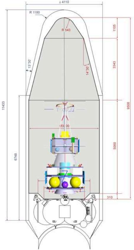
**Figure 7 :** Composite assembly of the two spacecraft for launch in a Soyuz fairing. The detector spacecraft is mounted on top of the heavier mirror spacecraft.
