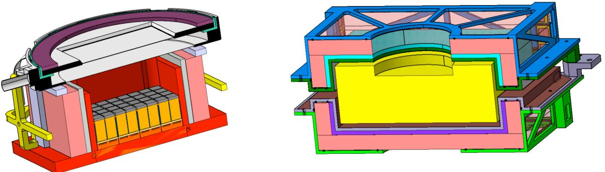
**Figure 4** : sketch of the detector assembly. Left : internal detectors system, cut-view, with Macro-Pixel Detector on top, the array of Cd(Zn)Te modules at the bottom, and the active and passive shielding walls on the sides. Right : the internal detector system (central volume) is surrounded by additional active and passive shieldings, in two halves.
