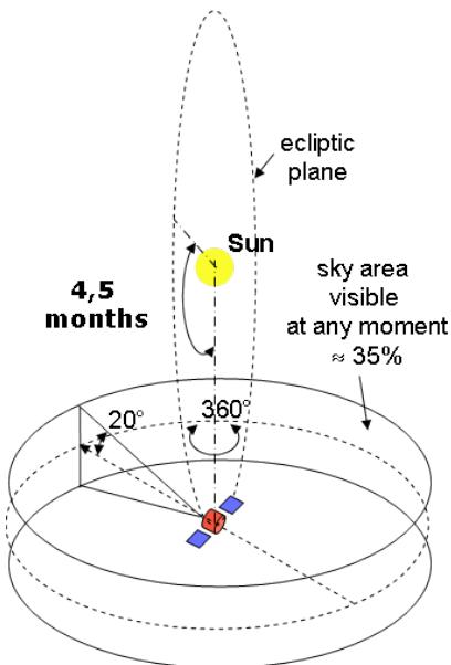
**Figure 5 :** Simbol-X viewing direction.
