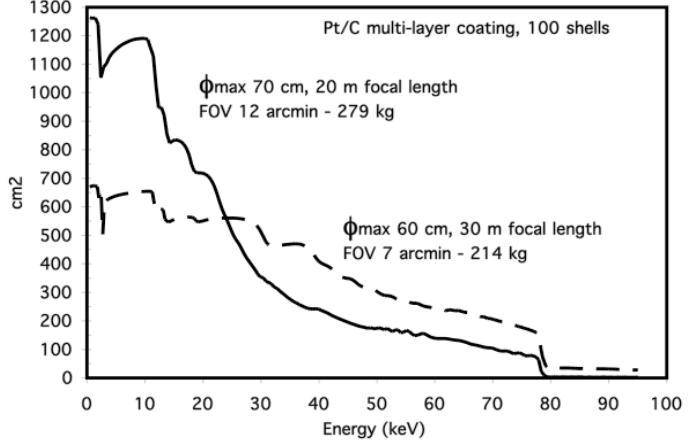
**Figure 2 :** Mirror effective areas for two study cases. Both are assuming a multi-layer coating. Characteristics are given in the figure.
