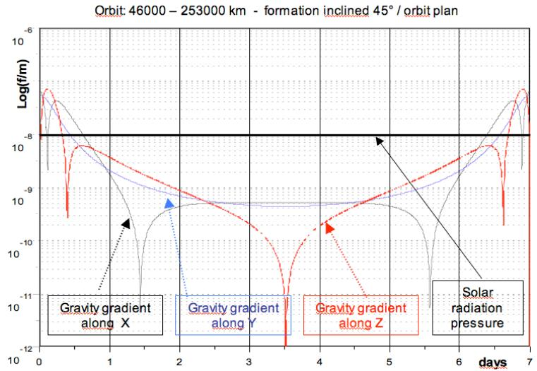
**Figure 6 :** Comparison of the solar radiation pressure with the gravity gradient along the 7 days of the Simbol-X orbit, for the 3 spatial axes.
