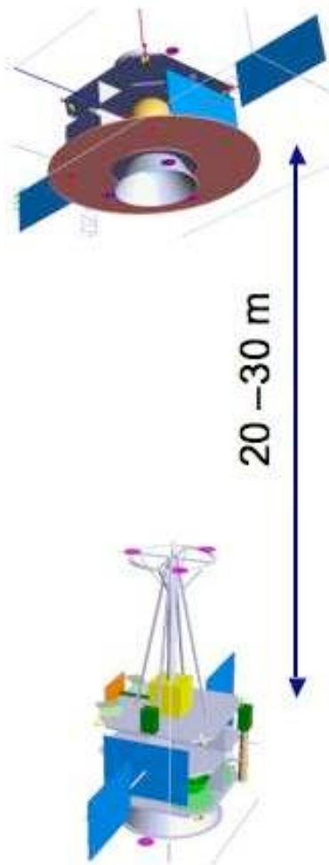
**Figure 1 :** Sketch (not to scale) of the Simbol-X configuration in flight, with mirror (top) and detector (bottom) spacecraft kept on a constrained formation. The focal plane unit has a  $\sim 1.5$  m collimator on top, while the mirror spacecraft carries a  $\sim 3$  m diameter circular sky baffle (see Section 3.3).
