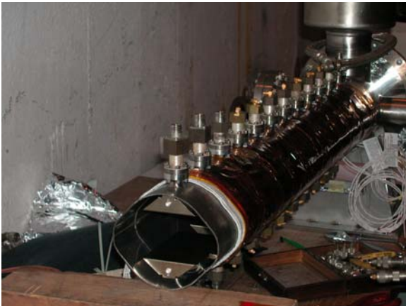
Figure 6 : Assembling of the vertical travelling wave PU.
