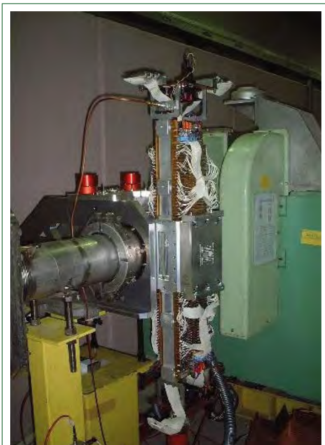
Figure 1. One of the KABES detectors moved horizontally 20 cm out of the beam line to see the entrance window.
