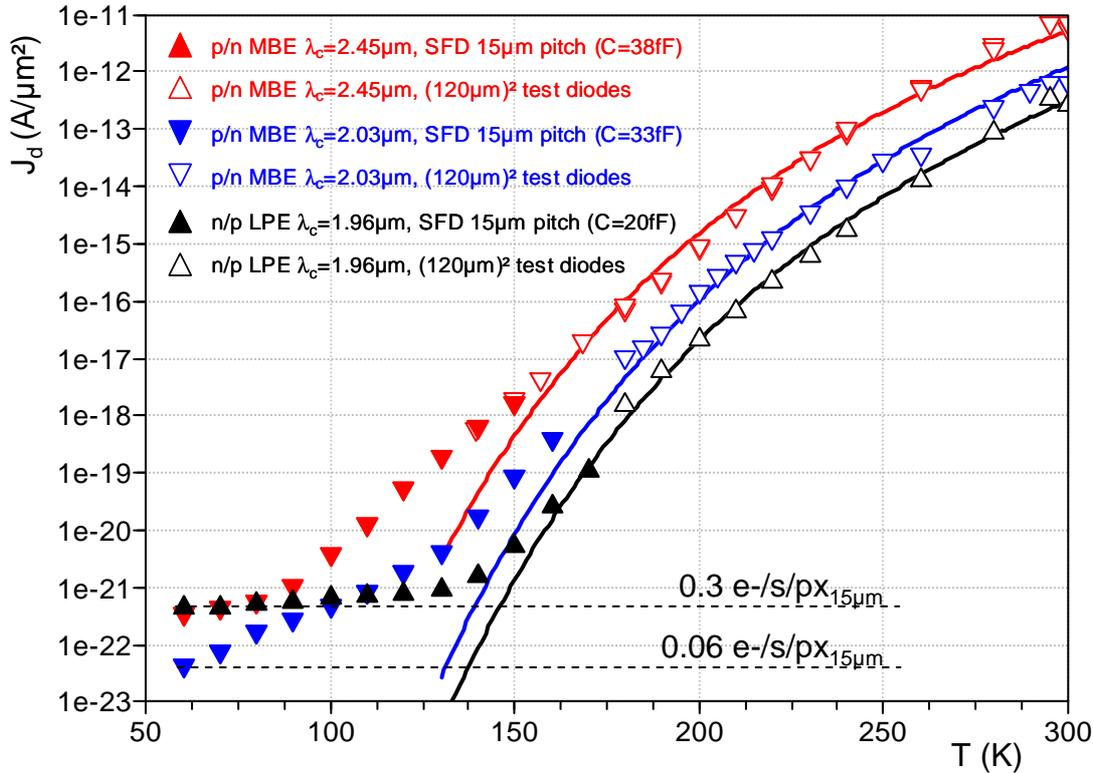
**Figure 10 : Dark current measurements carried out on PV3080 (red), PV3081 (blue), and PV3140 (black) using both SFD FPA and large test diodes.**
