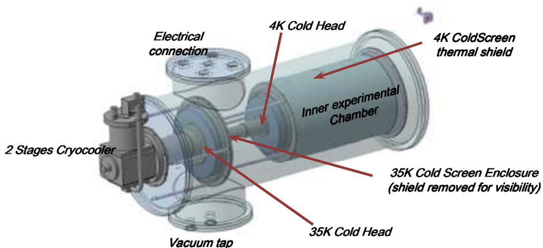
Figure 5: Light tight cryostat used with two stage cryo cooler.
