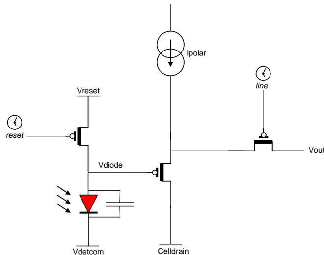
**Figure 4 : SFD pixel principle containing 3 MOS per pixel**
