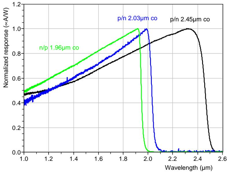
**Figure 1 : Example of spectral responses measured under high flux conditions using FTIR spectrometer at 110K**
