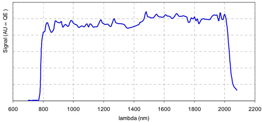
**Figure 2 : Example of spectral QE curve measured with a monochromator on layer PV3081 at 77K**
