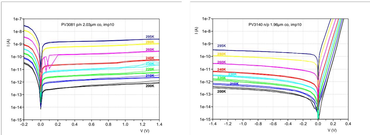
**Figure 3 : I(V) curves obtained at darkness between 200 and 300K for  $\sim 2\mu\text{m}$  co p/n and n/p diodes with  $10\mu\text{m}$  width squared implantation**
