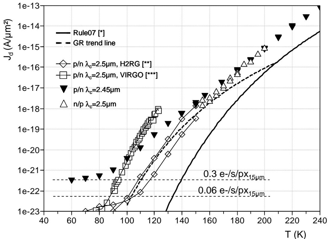
Figure 11 : measured dark currents and comparison with literature data at  $2.5\mu\text{m}$  cut-off [<sup>14, 16, 17</sup>]
