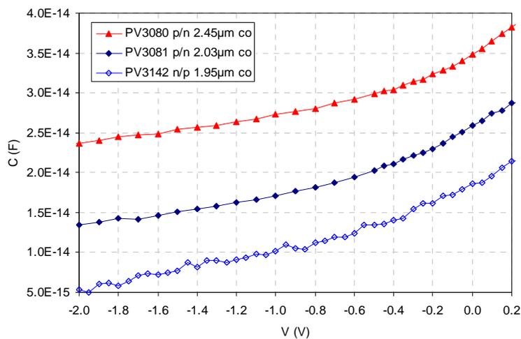
**Figure 7 : C(V) measurements at 77K carried out on test diodes.**
