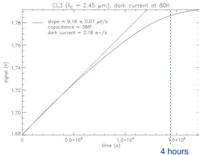
**Figure 8 : Typical integration ramp obtained at low temperatures**
