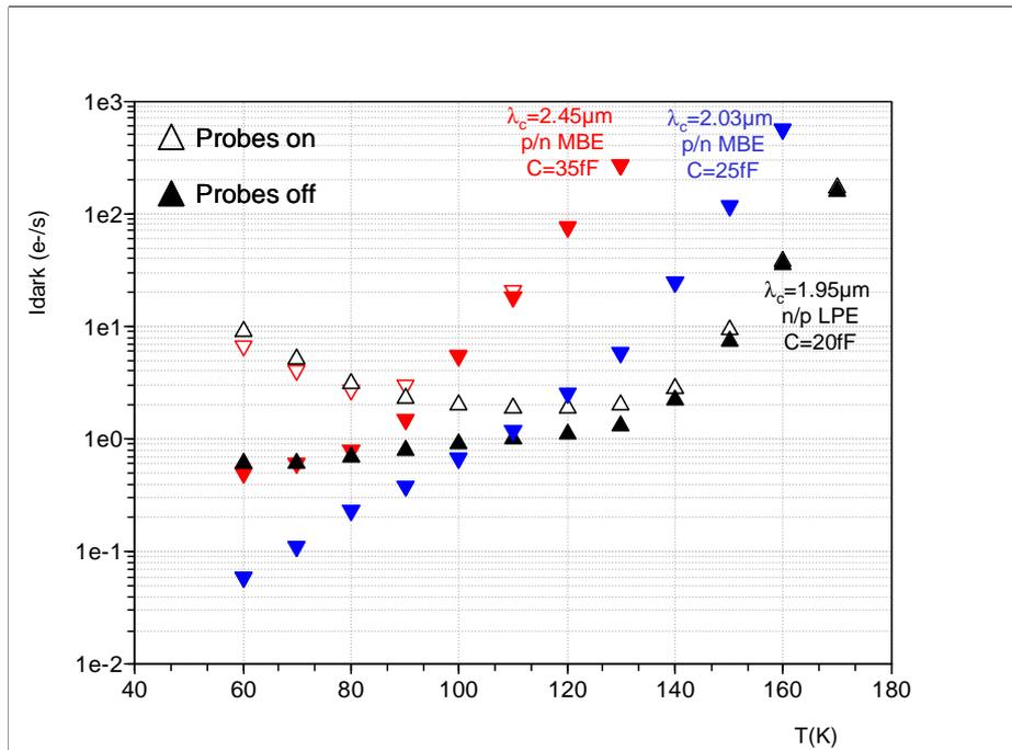
**Figure 9 : effect of additional temperature probes (2N2222) on the recorded dark current**
