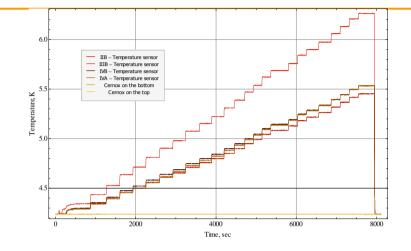
The change of temperature during the experiment in all monitoring sensors for the heated sample III
