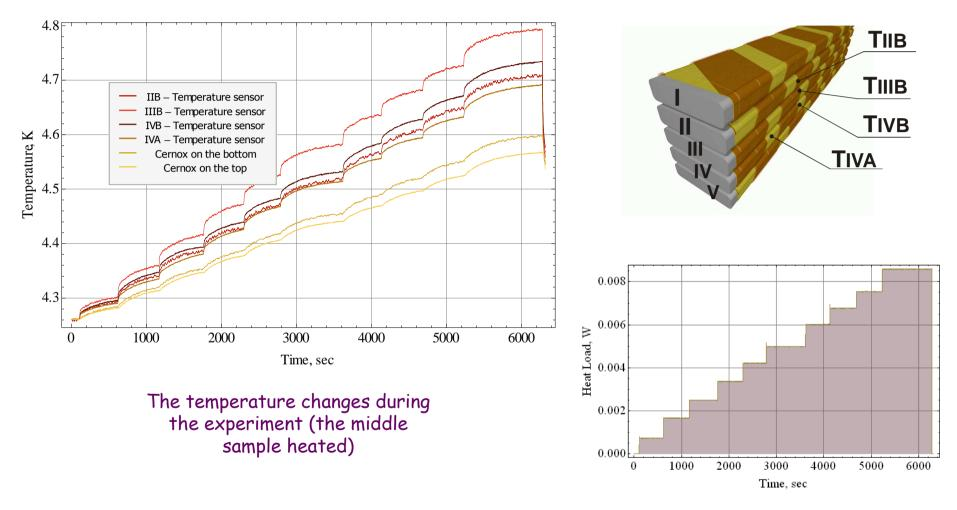
The heat dissipated during the experiment
