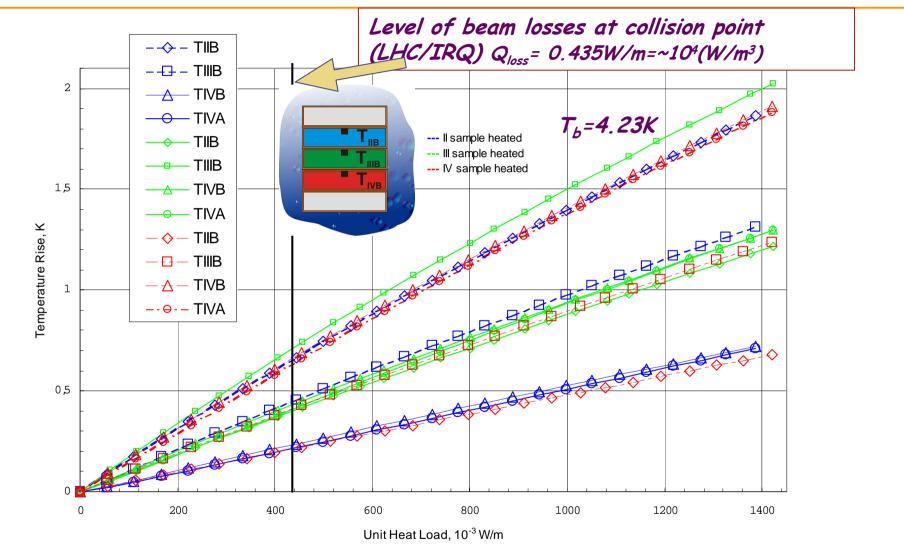
The temperature rise in the samples vs. unit heat load for the one heated sample
