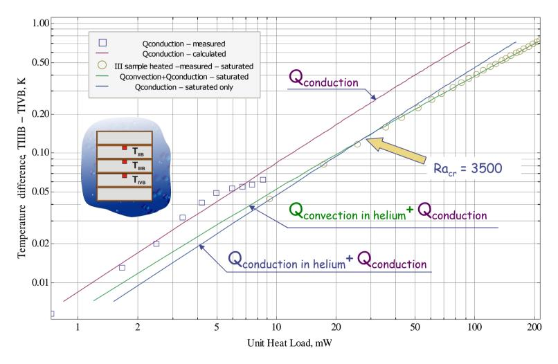
The comparison of measured and calculated heat transfer in saturated helium
