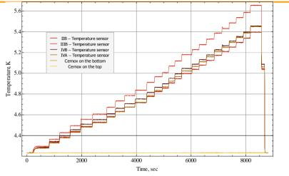
The rise of temperature for the three heated samples
