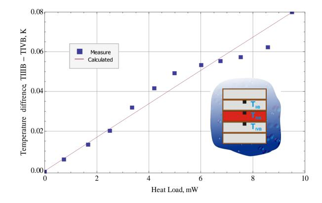
The calculated and measured differences of temperature between  $T_{IIIB}$  and  $T_{IVB}$  as the function of heat loaded to the sample III.
