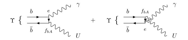
Amplitude for producing U proportional to gauge coupling
