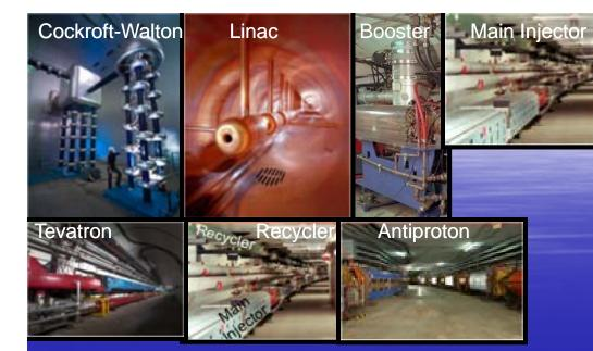
Unified control system for the entire complex •400 MeV Linac •8 GeV Booster Synchrotron •120 GeV Main Injector Synchrotron •1 TeV Tevatron Synchrotron •antiproton source - target/debuncher/accumulator •antiproton "Recycler" storage ring •fixed target lines
