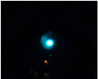
Electron spot coming from the electron gun on a phosphor screen
