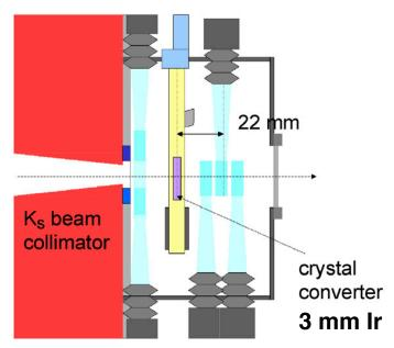
Pair-production enhancement from coherent interaction with crystal lattice was studied for AKS development Pair prod. enhancement vs  $E_{\gamma}$  and  $\theta_{\gamma}$  Moore et al., NIMB 119, 149 (1996)
