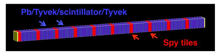
Thicker spy tiles (5-20 mm) with independent WLS fiber readout
