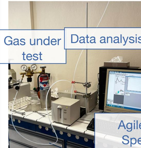
Agilent 8453 UV-visible Spectroscopy system
