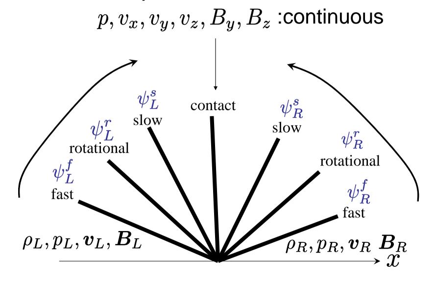
We solve the system of eqs. by Newton-Raphson method.  $W_L^s(\psi_L^s; U_L^r(\psi_L^r; U_L^f(\psi_L^f; U_L))) - W_R^s(\psi_R^s; U_R^r(\psi_R^r; U_R^f(\psi_R^f; U_R))) = 0$
