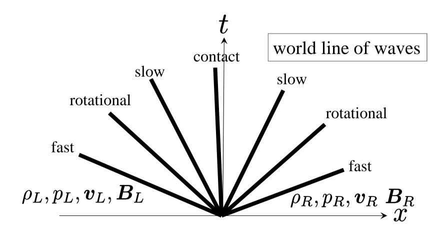
Determine the parameters associated with each wave so that the quantities other than density is continuous across the contact discontinuity.
