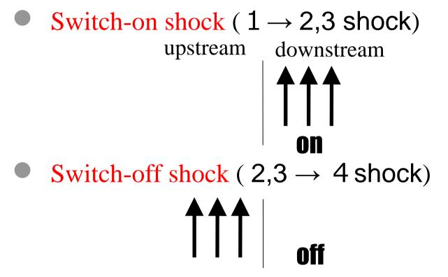
Switch-off shock lies at the boundary between the slow shock and intermediate shock
