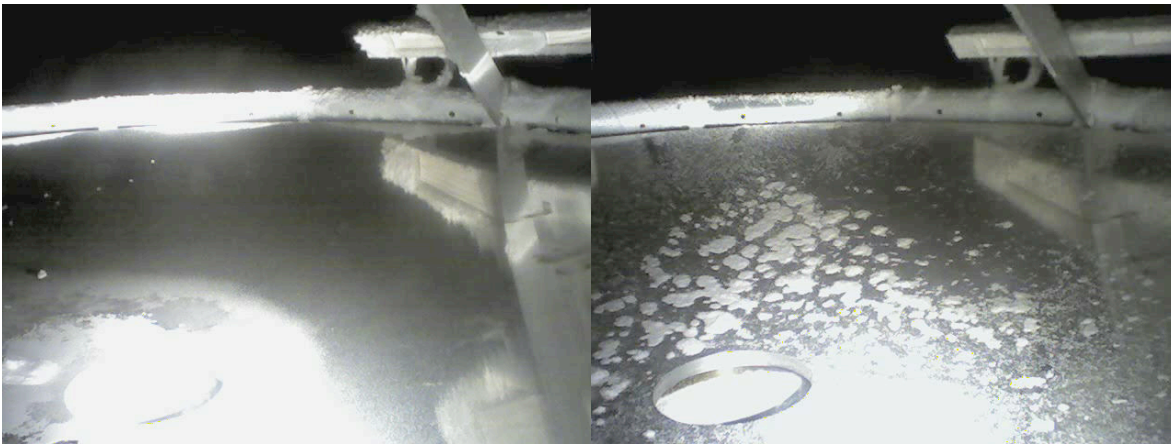
Figure 10: Left: On this web-cam photo, the mirror is heated 5°C above ambient. The snow is pushed toward the centre of the mirror by both gravity and the blower. Right: Without a cleaning anti-frost system, the mirror is rapidly covered with frost and snow.
