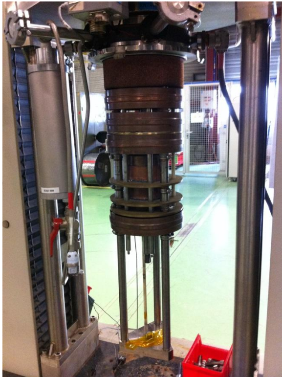
Cryostat supportant 5 tonnes
