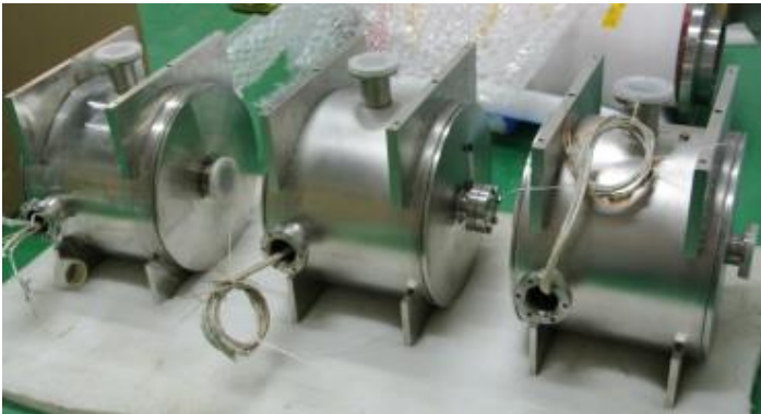
Three L150 solenoid has been finished and tested
