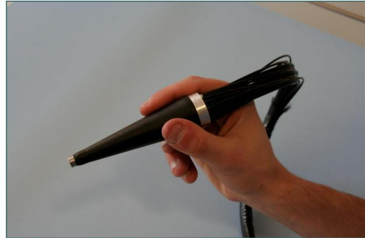
A first prototype was designed and constructed using multi-anode PMT; now, the use of SiPM is being pioneered.
