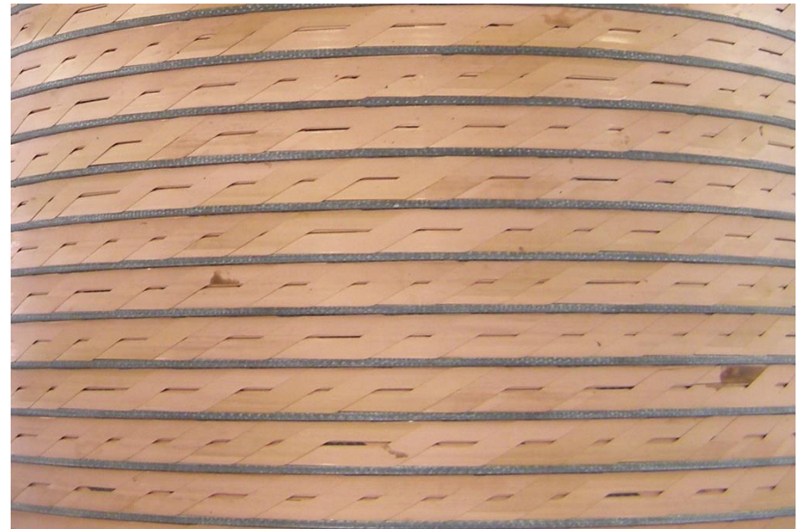
Roebel cable in low voltage winding
