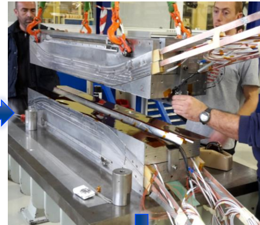
3. Assembly of 2 double-coils
