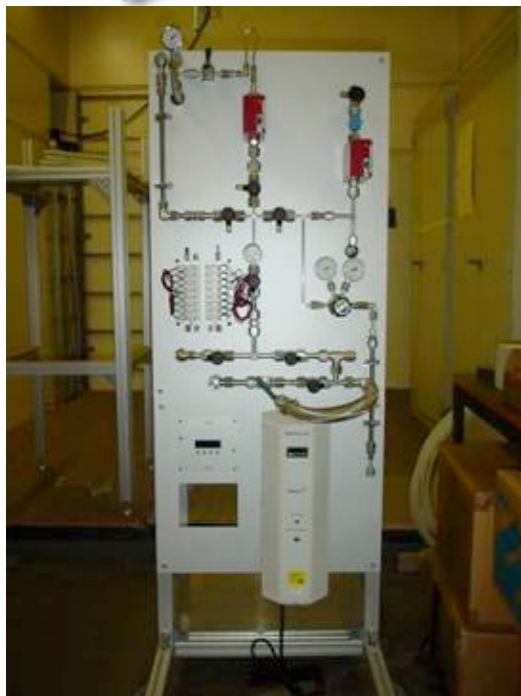
Metal heated getter H_2O , O_2 , N_2 , ... Diaphragm pump \sim 1L/h
