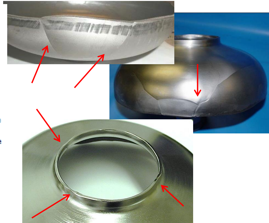
Figure 5. Elongation tests results for 3 single crystal samples with different orientations.
