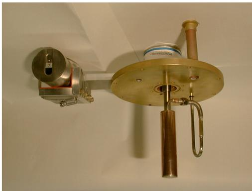
ARC Liquefier using BEI Tactical Cooler
