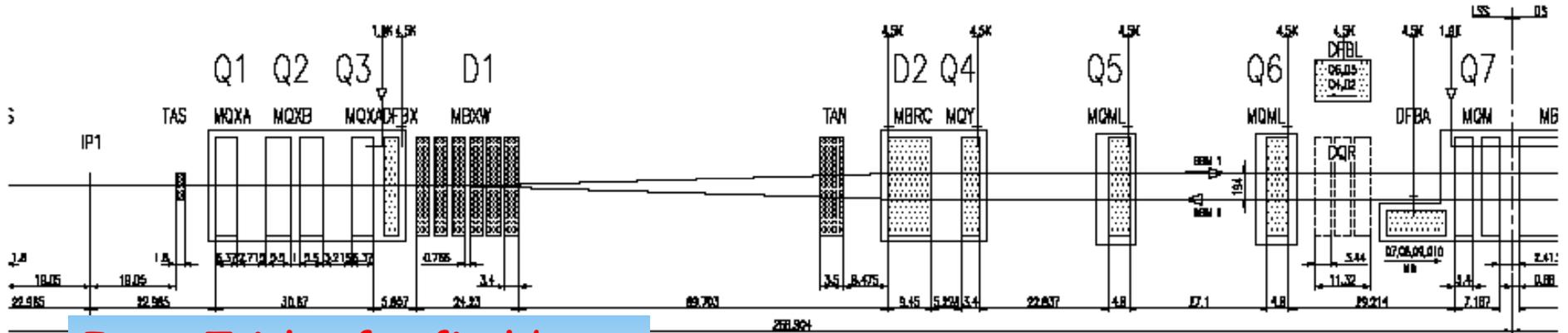
**Inner Triplet for final beam focusing/defocusing**
