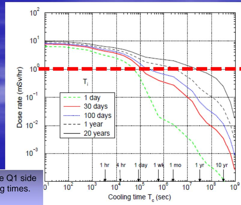
Averaged over surface residual dose rate (mSv/hr) on the Q1 side ( $z=2125\text{ cm}$ , bottom) of the TAS vs irradiation and cooling times.
