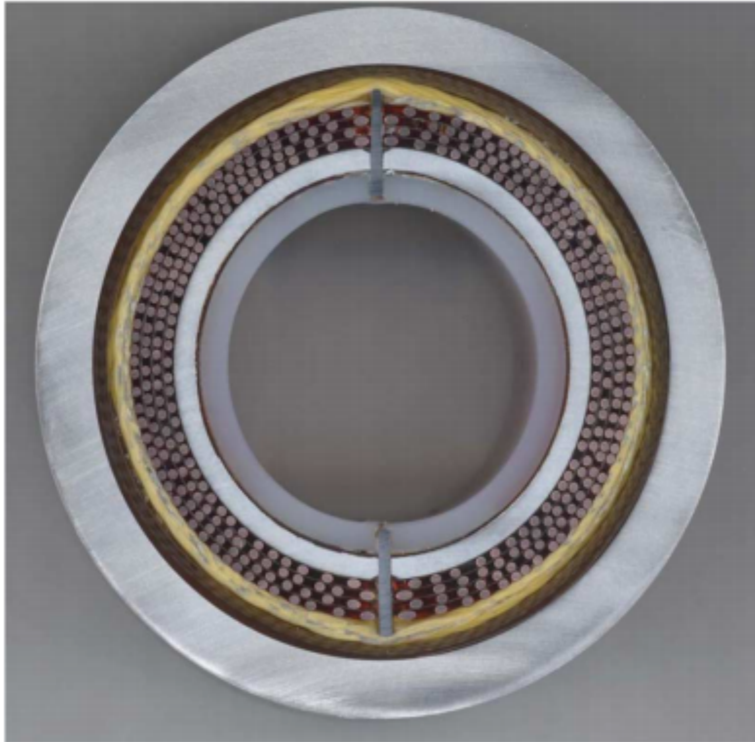
Fig. 8. Actual cross section of the dipole tested.
