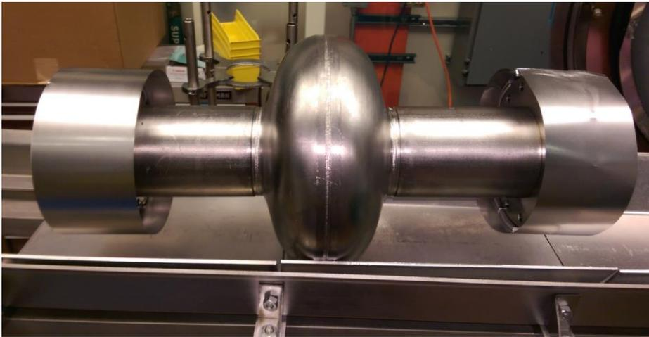
Protective caps and foils are BCP'd prior to every furnace cycle and assembled in clean room, prior to transporting cavity to furnace area
