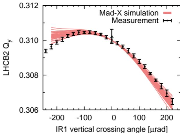
Octupole feed-down agrees with magnetic model of IR1, but not IR5
