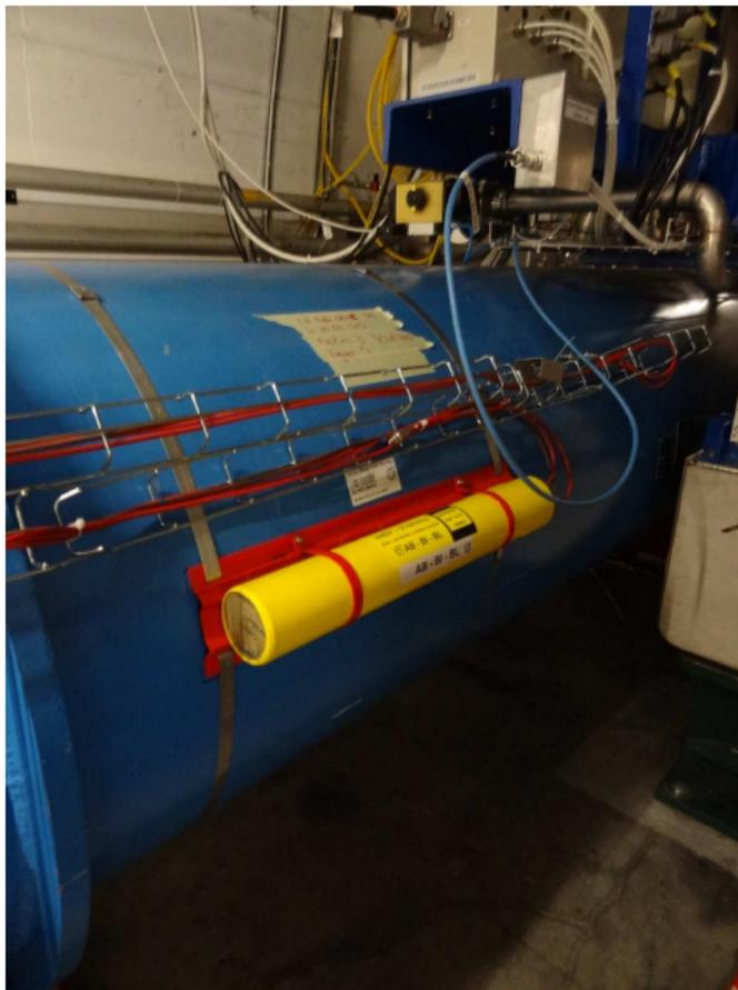
**Beam Loss Monitors (BLM) show losses at the vertical collimator**
