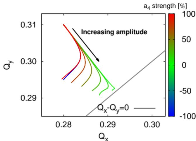
Model shows increasing closest approach with skew octupole ( $a_4$ ) strength
