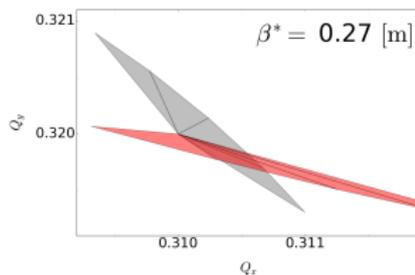
Potential for loss of Landau damping during  $\beta^*$  squeeze if IR- $b_4$  is not corrected
