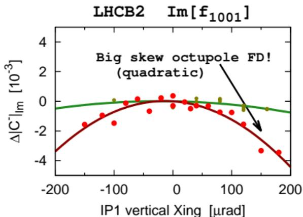
**Without correction crossing angle luminosity levelling could lead to loss of Landau damping**
