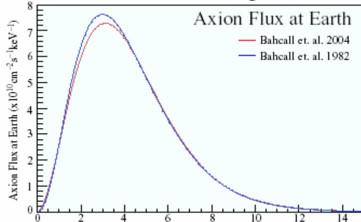
$$\Phi_a \approx 3.67 \times 10^{11} \text{ cm}^{-2} \text{ s}^{-1} \left( \frac{g_{a\gamma\gamma}}{10^{-10} \text{ GeV}^{-1}} \right)^2$$
