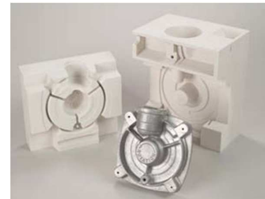
ZCast 3D Printed mold and cast aluminum part
