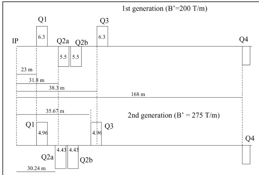
Same layout as present, but with larger-aperture and stronger final-focusing quadrupole magnets (Courtesy T. Sen)
