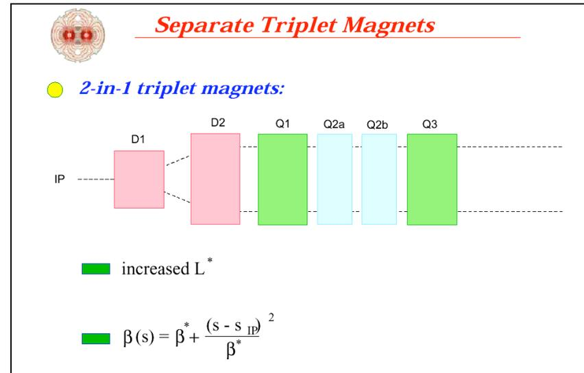
New layout where beam-separation dipoles are positioned in front of final-focusing quadrupole magnets (Courtesy O. Brüning)
