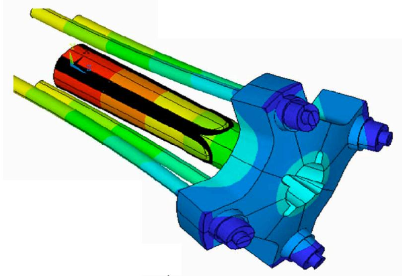
3-D model of US-LARP TQS01 at full energization (Courtesy S. CASPI, LBNL)
