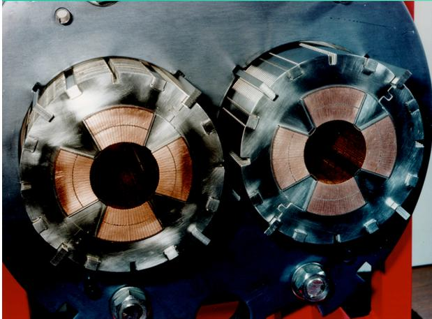
LHC arc quadrupole magnet
