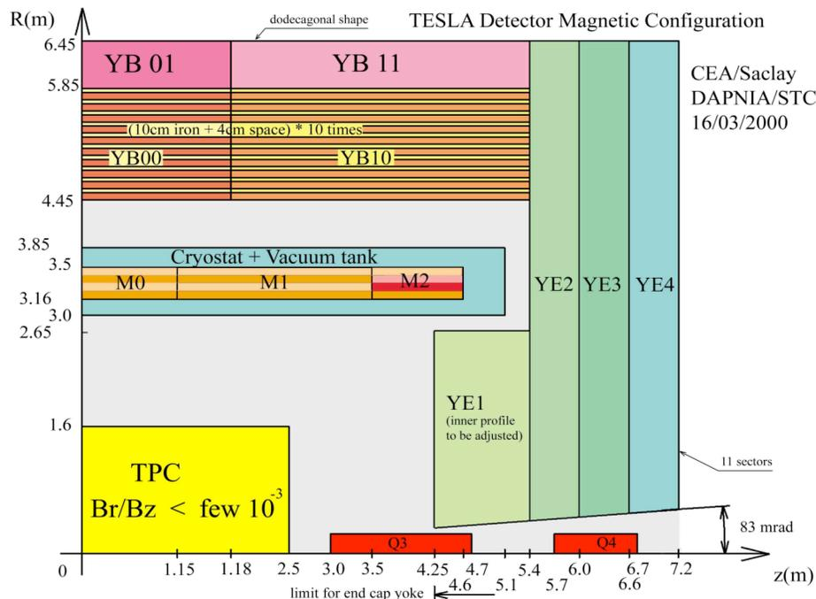
TESLA-type IR requiring LHC-type quadrupole magnets to be operated in a 4-T solenoidal background field (Courtesy F. Kircher)
