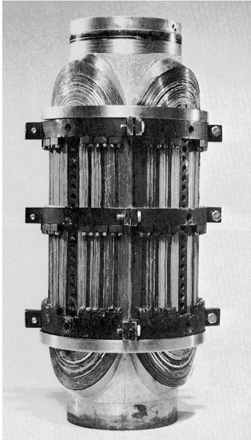
76-mm-aperture, 85-T/m quadrupole magnet model wound from Nb<sub>3</sub>Sn ribbons and cold tested at BNL in Jan. 1966 (Courtesy W.B. Sampson)
