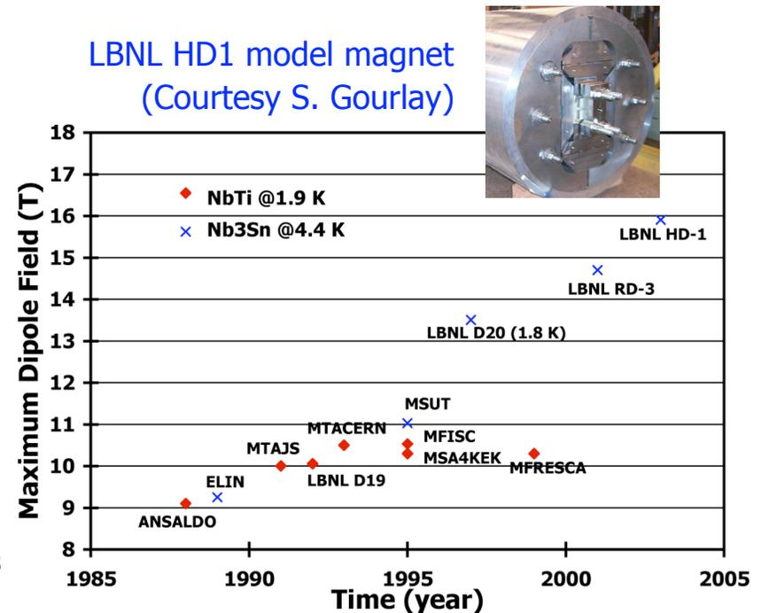
Progress on maximum quench field of dipole magnet models
