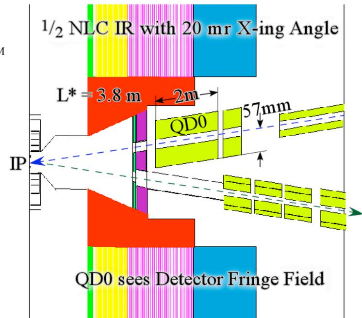
NLC-type IR with large crossing angle requiring strong but very compact quadrupole magnets to clear the way for crossing beam (Courtesy B. Parker)
