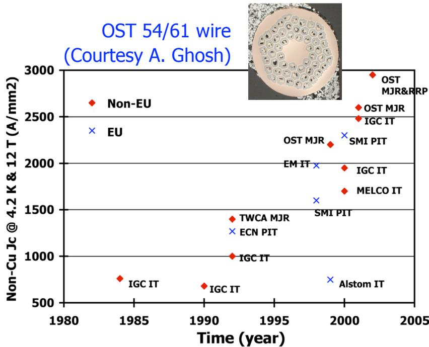
Progress on non-Cu J<sub>c</sub> (at 4.2 K and 12 T) of Nb<sub>3</sub>Sn wires
