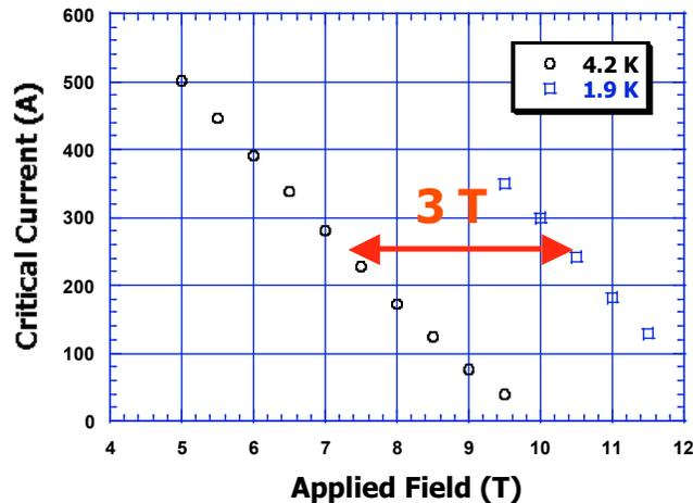
NbTi critical current enhancement from 4.2 to 1.9 K
