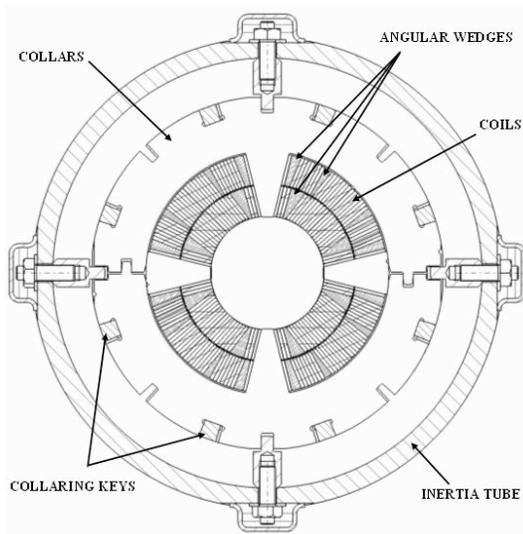
Cross-sectional view of CEA Nb<sub>3</sub>Sn quadrupole magnet model
