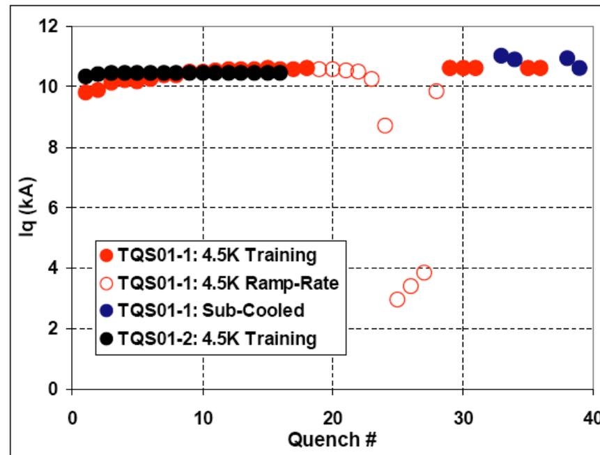
Cross-sectional view and training performance of US-LARP TQS01 quadrupole magnet model (Courtesy G. Sabbi, LBNL)
