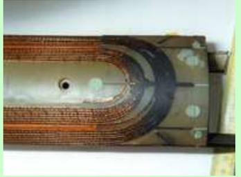
Insulated coil with mechanical cohesion
