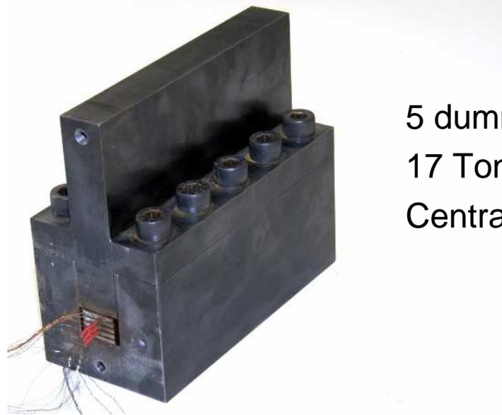
5 dummy stainless steel conductors stack
