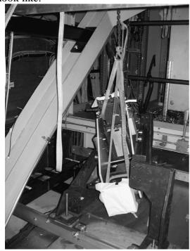
12/ Tighten the slings while bringing the detector upstream along the rails. Make sure the horizontal spacers are well
