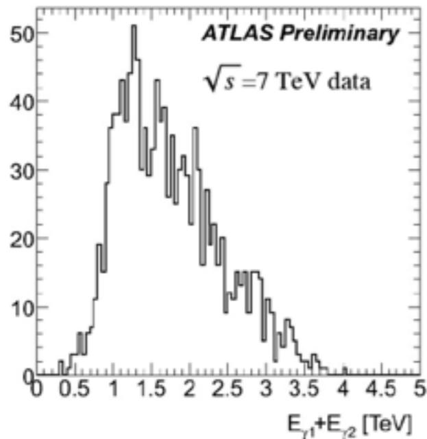
Energy distribution of 2 photon candidates in the ZDC, selected using the longitudinal shower profile. The ZDC energy scale was established using the endpoint measured in 7 TeV collision data. Since the shower energy is concurrently measured in the "pixel" coordinate readout channels this allows energy calibration to be established for these channels also.
