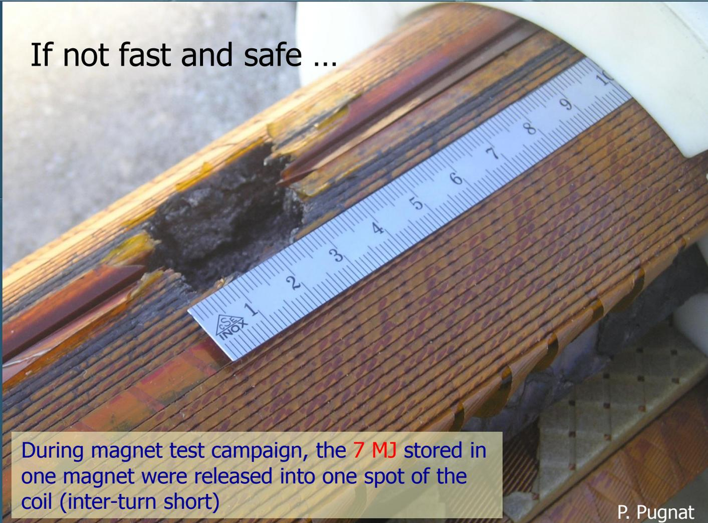
During magnet test campaign, the **7 MJ** stored in one magnet were released into one spot of the coil (inter-turn short)
