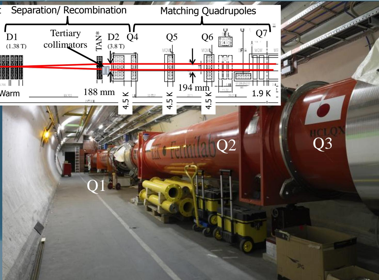
\* Protect Inner Triplet (TAS) and D2 (TAN) from particles coming from the IP
