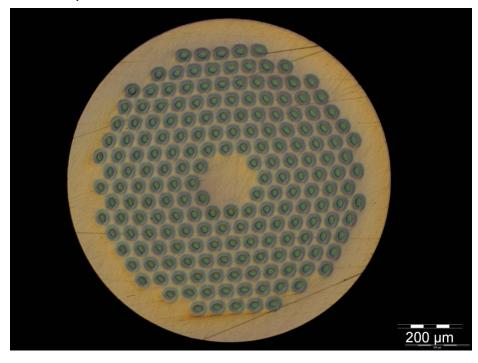
Work is on-going on a new strand architecture (169 stack) to reduce the filament diameter to 52  $\mu m$  at 1 mm strand diameter, and 35  $\mu m$  at 0.7 mm strand
