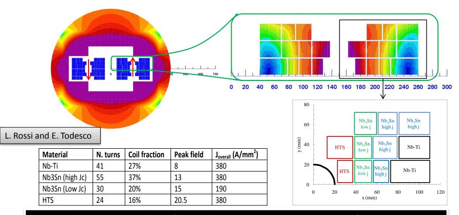
Magnet design: 40 mm bore (depends on injection energy: > 1 Tev)
