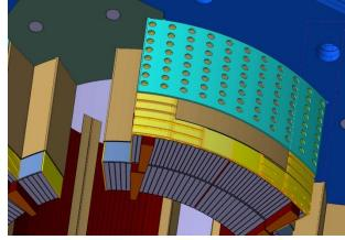
new insulation scheme, more porous in the coils and in the structure Higher heat removal (matching the gap to NbSn ?)
