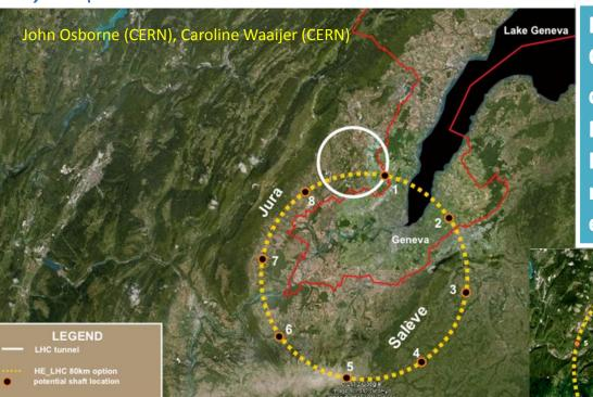
For a LEP300?, then for HE-LHC **Optimitation could be at 16 T field level:** collision energy 80 TeV c.o.m. Much better new infrastructure. However many costs go linearly, or more, with length. Magnet stored energy, beam energy also a concern
