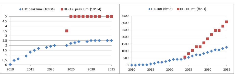
Figure 1.10. Left graph: peak luminosity for LHC with improving consolidation (diamonds) and with HL-LHC full performance (square markers). Right graph: the same for the integrated luminosity.
