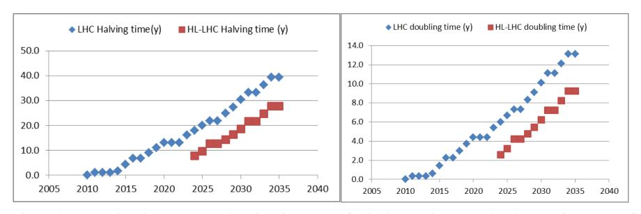
Figure 1.11 Halving time and doubling time for the LHC with improving consolidation and for HL-LHC with full performance.
