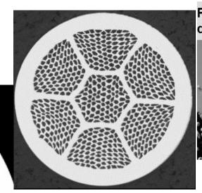
Porosity is still evident in densified wires
