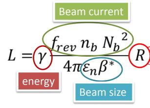
Beam current and emittance: involve Inj chain and whole ring β\* involve «only» 2 IRs, 600 m.
