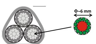
MgB<sub>2</sub> cable 6 kA at 20 K (> 12 kA at 4.5 K)
