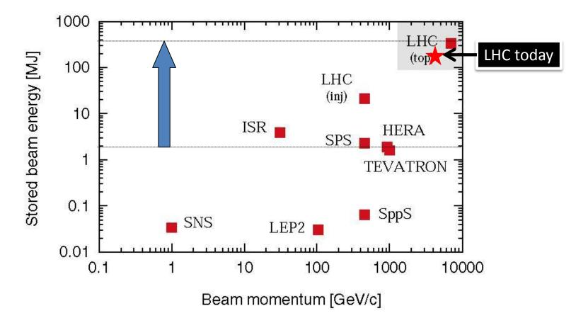
At less than 1% of nominal intensity LHC enters new territory. Collimators must survive expected beam loss...
