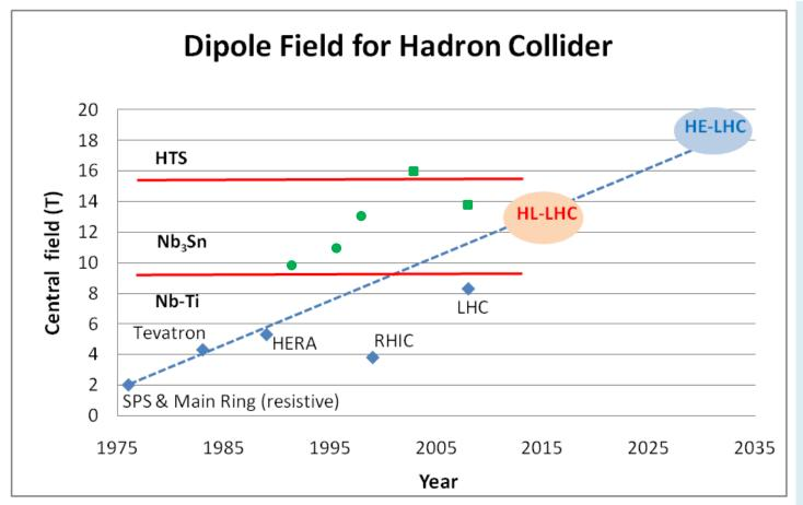
Looking at performance offered by practical SC, considering tunnel size and basic engineering (forces, stresses, energy) the practical limits is around 20 T. Such a challenge is similar to a 40 T solenoid (μ-C)
