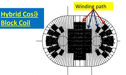
• Beam bore diameter – 40 mm
