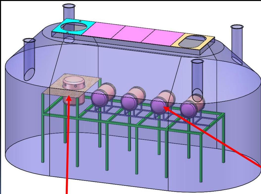
To achieve an extremely low background environment, use ultrapure water contained in a large SS water tank with 25(l)x13(w)x13(h), 3400 ton capacity
